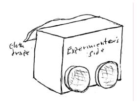
Sleeves constructed of 14 x 18 mesh brass screen
